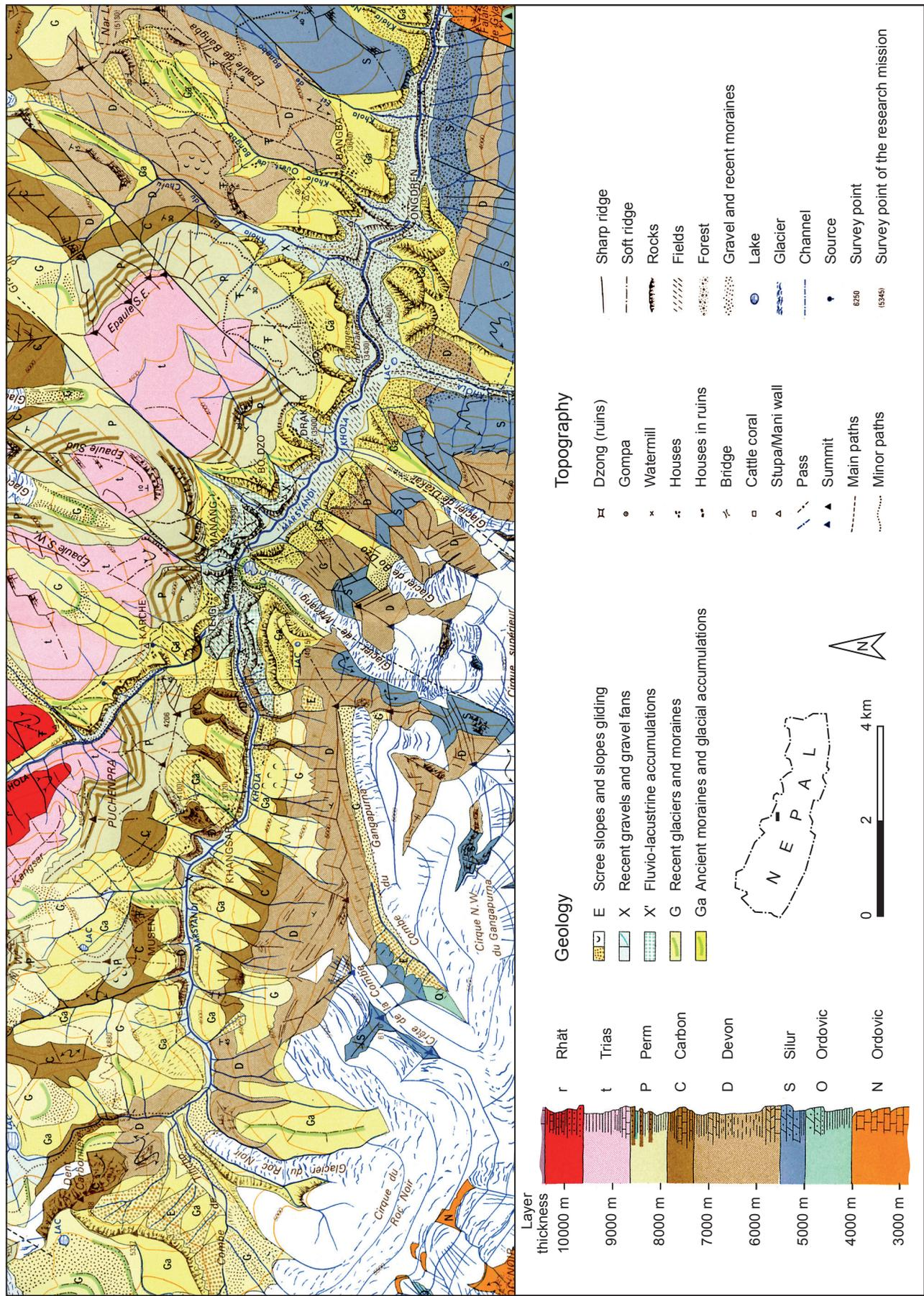
Fig. 6.19: Geological map of Manangbhot showing the vast extension of moraines and fluvio-glacial sediments. Modified from geological sketch map of Nyi Shang (Bordet et al., 1975). More recent work (Weidinger, 2006) has shown that the origin of the majority of this material is a large rockslide which is partially overlain by moraines.
